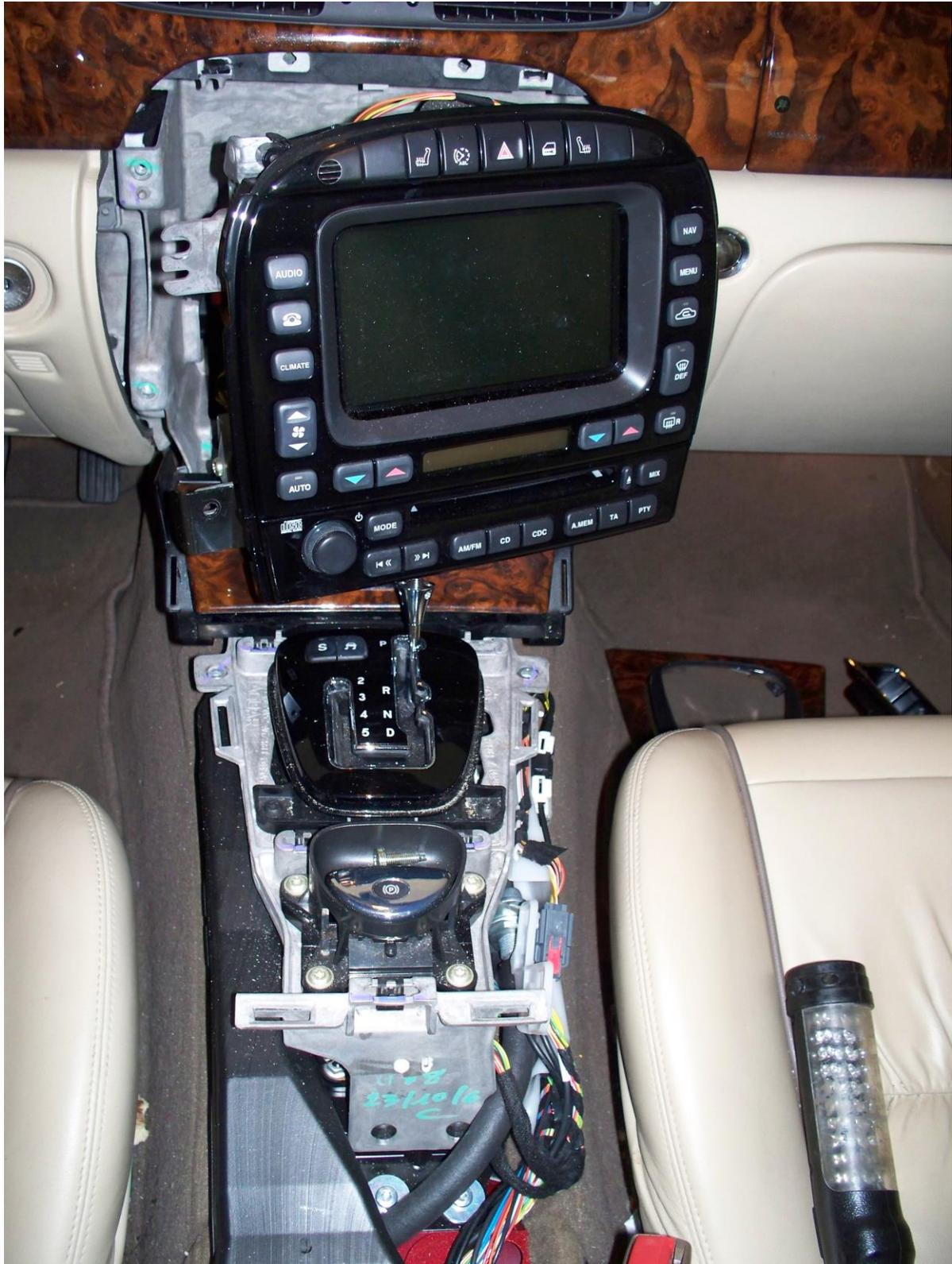
Now you can slide the head unit out. No need to disconnect it all. The radio connector is on the left side rear of the lower head unit.
